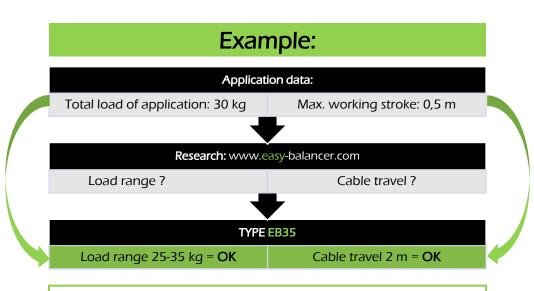
Make sure, that the load to be balanced is within the load range of the product, while the working stroke should be less than the maximum cable travel.
